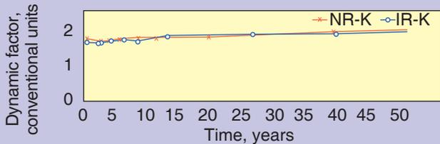
**Figure 5 - modification of the hysteresis of rubbers based on natural rubber (NR-K) and the combination of synthetic isoprene and synthetic cis-butadiene rubber (IR-K) over time**
