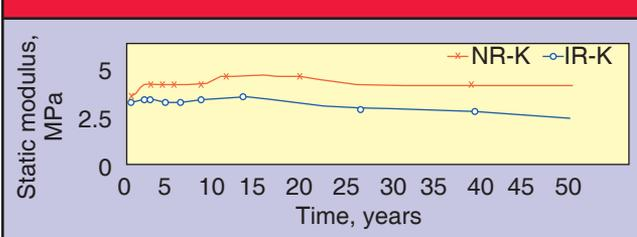
**Figure 2 - modification of the dynamic modulus of rubbers based on natural rubber (NR-K) and the combination of synthetic isoprene and synthetic cis-butadiene rubber (IR-K) over time**
