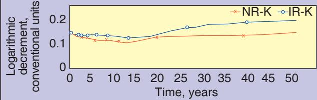
**Figure 3 - modification of the dynamic factor of rubbers based on natural rubber (NR-K) and the combination of synthetic isoprene and synthetic cis-butadiene rubber (IR-K) over time**
